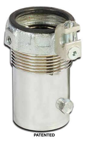
Slide on coupling with 5 female threads receive conduit or connectors and 10 male threads for two lock nuts and a ground bushing also available.
