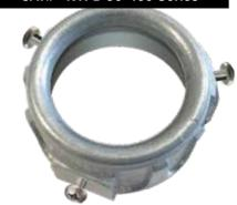
Rounded edge prevents damage to wire during pulls Saves time when pulling branch & feeder wire Serrated edge on under side of bushing serve as locknut Split plastic bushing also serves as locknut Install one with every connector
