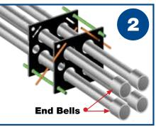
2. Ream out conduits and glue on end bell adapters to each conduit inside or outside manhole or vault
