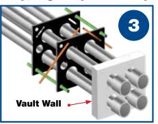
3. Slide conduits with bell end adapters thru manhole openings inside or outside manhole or vault
